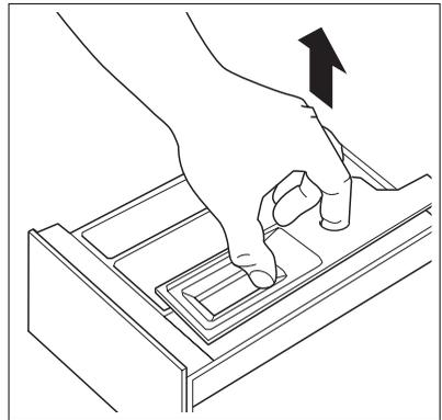
3. Having removed the drawer, use a small brush to clean the recess, ensuring that all washing powder residue is removed from the upper and lower part of the recess.
